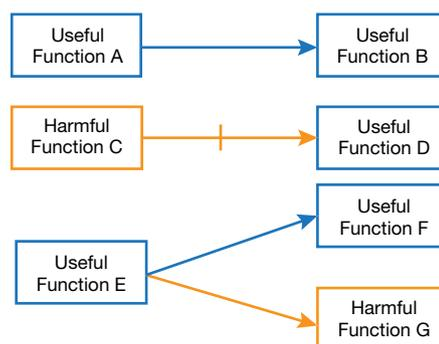
▲ **Figure 2.** The FAST diagram can be modified to make it easier to understand. Useful functions are outlined in blue, while harmful functions are outlined in orange. Moving against the direction of the arrow ask “how?” Moving in the direction of the arrow ask “why?”
