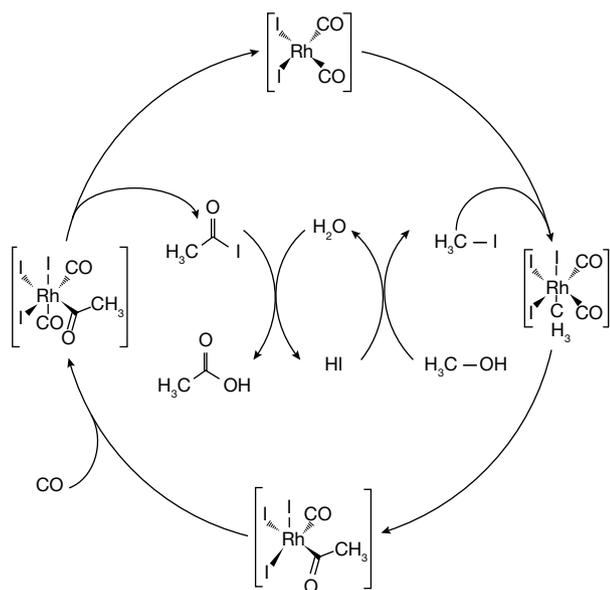
▲ **Figure 3.** Acetic acid is produced by the catalytic carbonylation of methanol.
