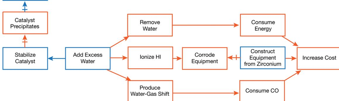
▼ **Figure 6.** The useful function “Add Excess Water” produces the useful function “Stabilize Catalyst,” but it also produces three harmful functions: “Remove Water,” “Ionize HI,” and “Produce Water-Gas Shift.” The function “Add Excess Water” is said to be in contradiction because it produces both useful and harmful functions.
