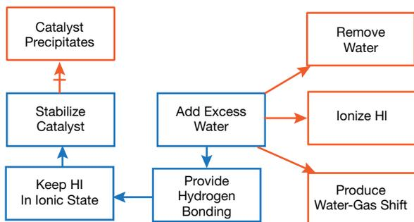
▲ **Figure 7.** Expanding the function model shows how water stabilizes the catalyst. The hydrogen bonding properties of water keep hydrogen iodide in an ionic state.
