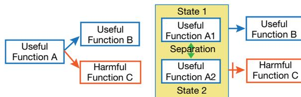
▲ **Figure 8.** Contradictions are resolved by separating the function that produces the contradiction (Function A) into two states. In State 1, the useful result (Function B) is produced, and in the State 2, the harmful effect (Function C) is counteracted.
