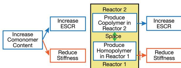
▲ **Figure 9.** Increasing the concentration of comonomer in a high-density polyethylene copolymer improves the environmental stress crack resistance (ESCR). However, the increased comonomer also reduces polymer stiffness. The use of two reactors resolves the contradiction between the high-density polyethylene copolymer's stiffness and its resistance to environmental stress cracking.
