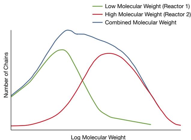
▲ **Figure 10.** HDPE copolymer produced in two reactors has a bimodal molecular weight distribution, representing a separation in structure.
