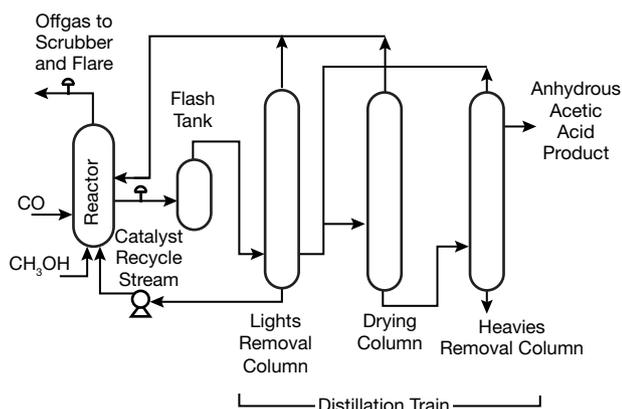
▲ **Figure 4.** The methanol carbonylation process uses a reactor, a flash tank, and three distillation columns to produce anhydrous acetic acid.
